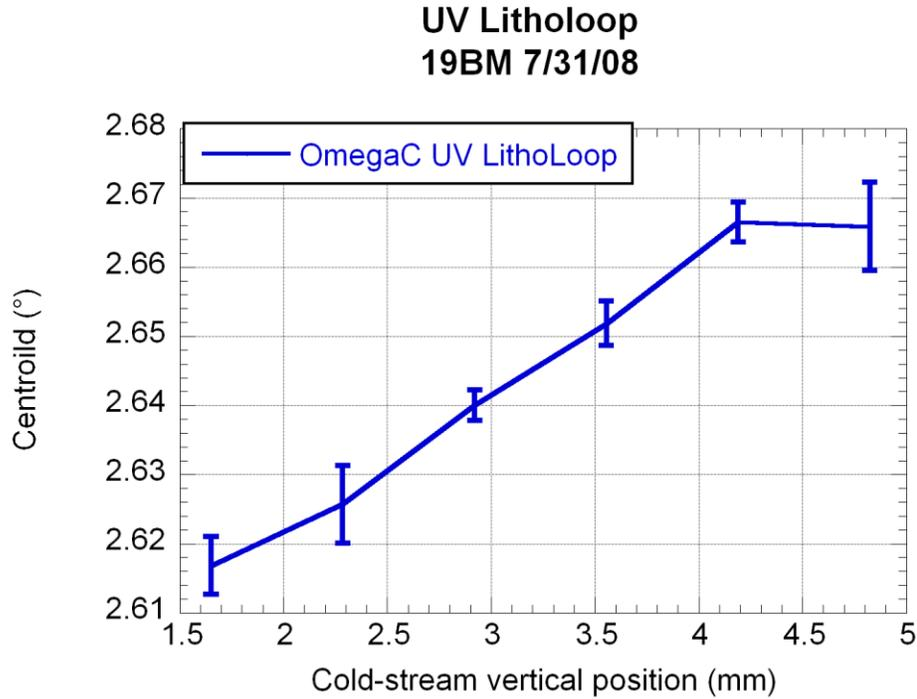
Figure 3. Angular centroid positions vs. cold-stream position. Error bars indicate movement of the reflection centroid but not how the profile may be changing.
