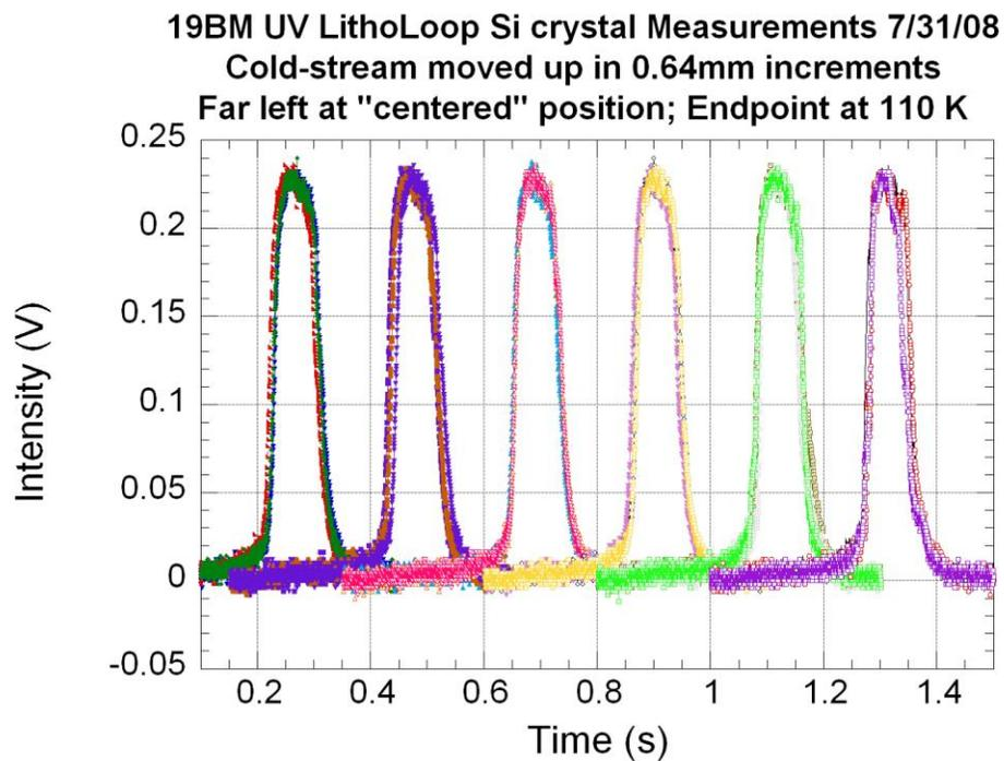
Figure 1. Peak profiles at different cold-stream positions. Force increases from left to right.
