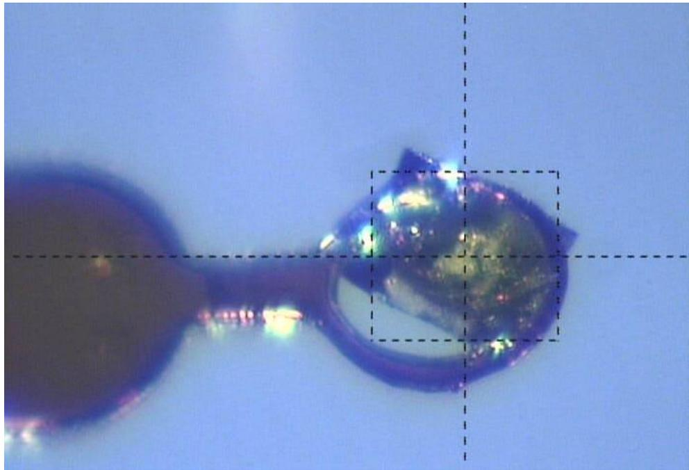
Photo 2. Bottom camera view of the sample looking at the back of the loop directly up into the crystal. The crystal and loop are oriented perpendicular to cold-stream.
