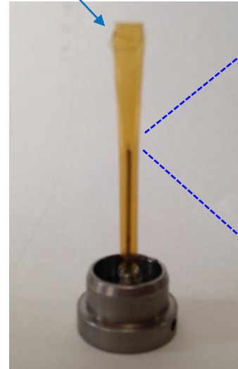
SPIKA LB grade with SPINE Cap Tube diameter=3.0mm Tube thickness=20 \mu m
